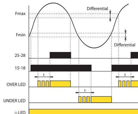
After the supply (monitored) voltage is connected, the green LED is on. If the value of the monitored frequency falls within the range between the two set levels Fmin - Fmax no red LED is on. The relay UNDER is triggered (contacts 15-16-18) and the relay OVER is disconnected (contacts 25-26-28).
