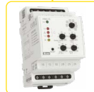
HRN3-70 Adjustable range (190-500 V), asymmetry (2-10 % +OFF), undervoltage (80-95 % from the range), restart delay (1-300 s), selectable memory, 2x output contact, TRUE RMS. page 38
