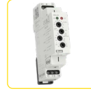
HRN-39, HRN-39/2 Multifunction, supply and monitored voltage in range of AC/DC 24-150 V, 1x (HRN-39) / 2x (HRN-39/2) output for Umax and Umin with adjustable levels. page 33
