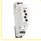
HRN-31, HRN-31/2 Multifunction, supply and monitored voltage in range of AC/DC 48-276 V, 1x (HRN-31) / 2x (HRN-31/2) output for Umax and Umin with adjustable levels. page 33
